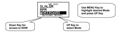
**KDW Adjustable Pull Parameter** – This background setting allows you to tailor the pull characteristics. To access, highlight Menu Key D, and press the DOWN Key to access this KDW screen:
