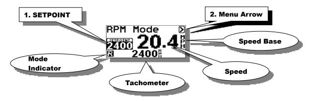
Operating in this mode is very similar to using the Wakeboard or Trick modes, except the system is now controlling to an RPM **SETPOINT**.
