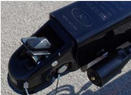
The coupling should not be allowed to lay on the ground where dirt or sand can enter the socket. This can cause excessive wear when the trailer is towed again, or it can cause the locking mechanism to jam.
