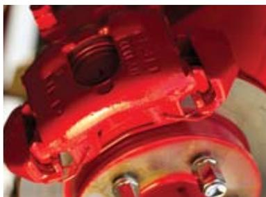
Your MasterCraft trailer brakes are designed to operate automatically when the tow vehicle's brakes are applied. These are known as surge brakes. When the tow vehicle slows down or stops, the forward momentum (surge) of the trailer against the hitch ball applies pressure to a master cylinder in the trailer coupler. This pressure activates the trailer brakes through a hydraulic system, much like the brakes on your automobile.
