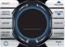
In normal mode the up/down buttons control volume. In FOLDER mode it will toggle through folders and songs.
