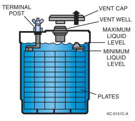
Figure 4-9. Battery Level
