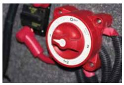
Figure 4-10. Battery Switch
