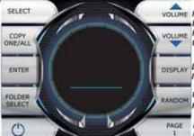
VOLUME In normal mode the up/down buttons control volume. In VOLUME FOLDER mode it will toggle through folders.
