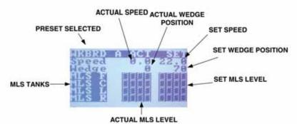
The cruise speed screen will show the normal information along with the preset that has been selected. You can reset the presets to factory defaults in the setup screen.
