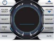
NOLUME In normal mode the up/down buttons control volume. In FOLDER mode it will toggle through folders and songs.
