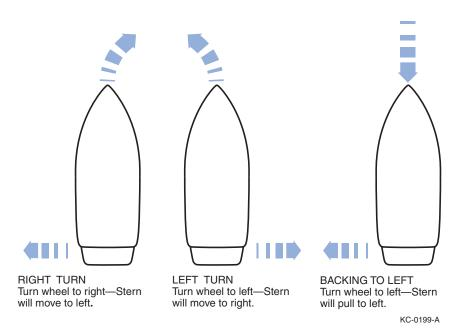
Figure 3-8. Turning with a Rudder
