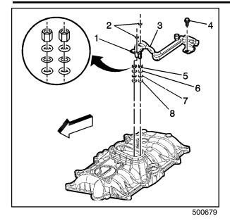
17. Remove the fuel pipe bolt (4).
