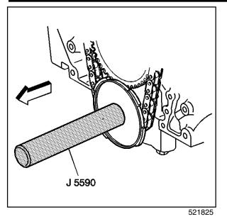
**Important:** Align the keyway on the crankshaft position sensor reluctor ring with the woodruff key (crankshaft balancer) in the crankshaft, and install the crankshaft position sensor reluctor ring onto the crankshaft until completely seated against the crankshaft sprocket.
