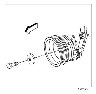
2. Remove the bolts and the crankshaft pulley.
