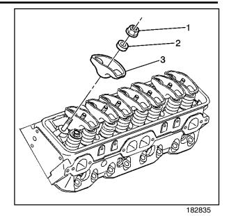
2. Remove the valve pushrods.
