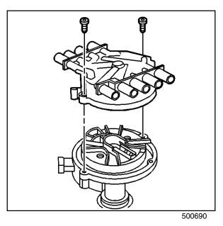
4. Install a NEW distributor gasket onto the distributor.
