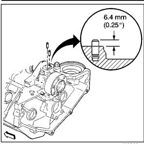
6. Inspect the pins (oil pump locator) for damage, replace the pins if required.
