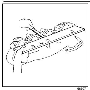
4. Measure the alignment or surface flatness of the exhaust manifold flanges using a straight edge and a feeler gauge. Refer to *Engine Mechanical Specifications.*
