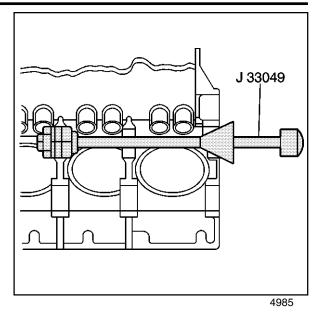
5. Carefully remove the J 33049 from the engine block.
