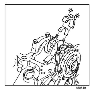
Important: Place matchmarks or numbers on the connecting rods and the connecting rod caps.
