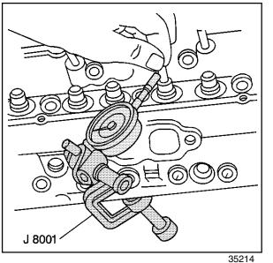
10. Measure the valve stem-to-guide clearance.
