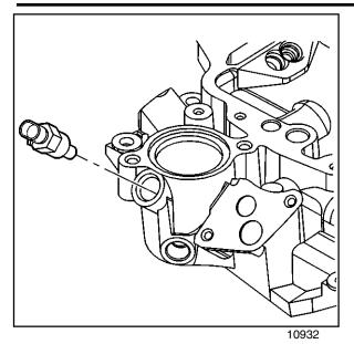
12. Remove the engine coolant temperature (ECT) sensor from the lower intake manifold.
