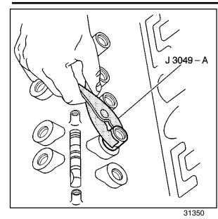
**Important:** Some valve lifters may be stuck in the valve lifter bores because of gum or varnish deposits and may require the use of *J 3049-A* for removal.
