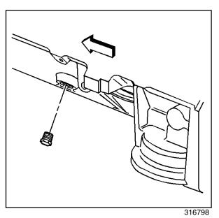
3. Remove the engine block coolant drain hole plug and allow the coolant to drain into a suitable container.
