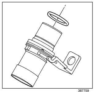
**Important:** Always install a NEW crankshaft position sensor seal (O-ring) during assembly.
