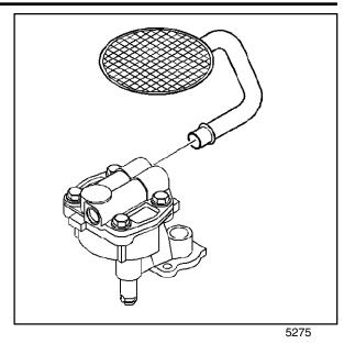
3. Remove the oil pump cover bolts.
