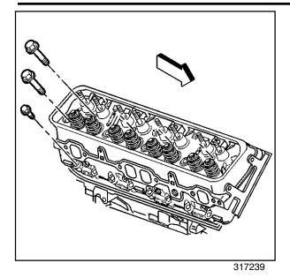
2. Remove the cylinder head bolts.
