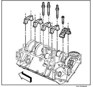
4. Install the crankshaft bearings into the crankshaft bearing caps.
