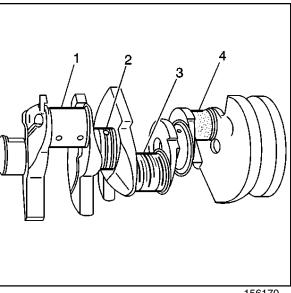
6. Inspect the crankshaft balancer key (1), the keyway (2) and the threaded hole (3) for damage.
