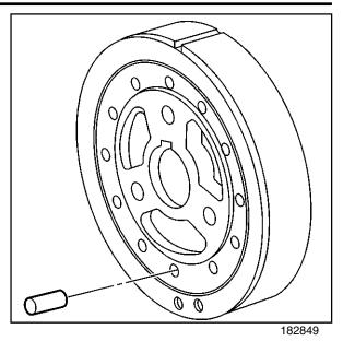
*Notice:* The inertial weight section of the crankshaft balancer is assembled to the hub with a rubber type material. The correct installation procedures (with the proper tool) must be followed or movement of the inertial weight section of the hub will destroy the tuning of the crankshaft balancer.
