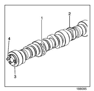
Important: If any camshaft bearing is excessively worn or scored, replace all the camshaft bearings.
