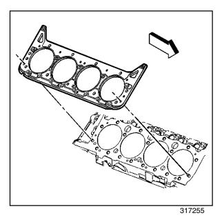
4. Remove and discard the cylinder head gasket.
