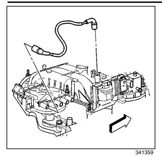
14. Install the ignition coil wire harness.
