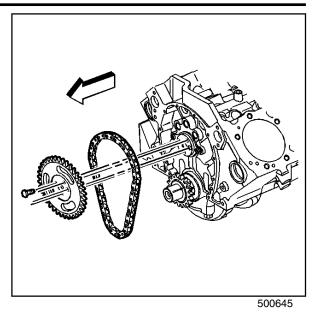
**Important:** Do not use a hammer to install the camshaft sprocket onto the camshaft. To do so may dislodge the expansion cup plug (camshaft rear bearing hole) and/or damage the camshaft.
