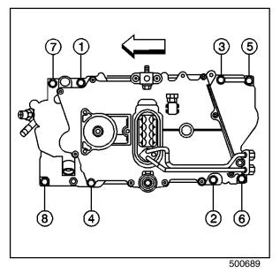
5. Install the lower intake manifold onto the engine block.
