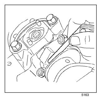
8. After the piston and connecting rod assemblies have been installed, then lightly tap each connecting rod assembly (parallel to the crankpin) in order to ensure that the connecting rods have side clearance.
