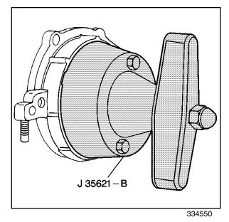
13. Install the J 35621-B onto the rear of the crankshaft and hand tighten the tool bolts until snug.
