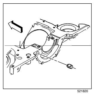
2. Remove the S type pin (crankshaft rear oil seal housing)(if required).
