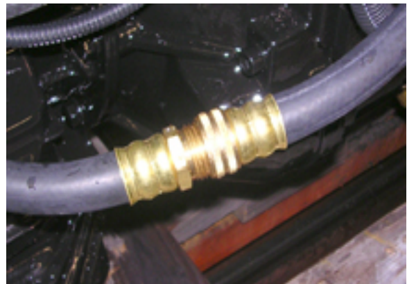
Separate Exhaust Manifold Drains
