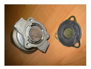
5. Install top cover with rubber seal over impeller assembly and install 3 bolts and lock washers tight to seal.
