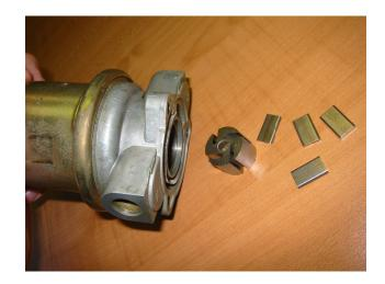
4. Remove screen filter inside pump body by gently lifting straight out or upwards.
