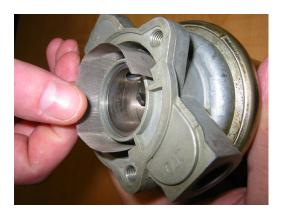
2. Insert impeller body (center slot down) into pump body.
