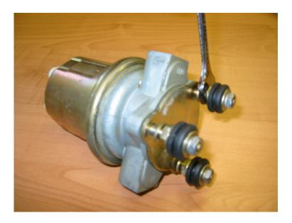
2. Remove the top cover plate, rubber seal and metal disc from atop the impeller assembly.
