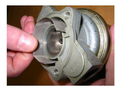
5. Clean impeller body, 4 vanes, screen filter and inside of pump body chamber of all varnish, gum and trash with carburetor cleaner or other suitable cleaning solvent.
