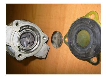
3. Remove impeller and 4 vanes from pump by inverting pump and tapping pump body gently. (NOTE: vanes and impeller should fall freely from pump body. Varnish and gums formed by gasoline breakdown may cause impeller and vanes to stick inside pump body. Tapping the pump body should free impeller and vanes to fall out.)
