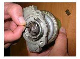
4. Insert metal disc on top of impeller assembly.
