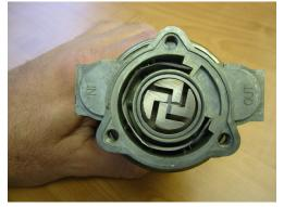
3. Insert the 4 impeller vanes into impeller body slots and insure that each vane is free to move outward within their slots by centrifugal force. (NOTE: both sides and edges of impeller vanes are interchangeable and can be reassembled with either edge out.)
